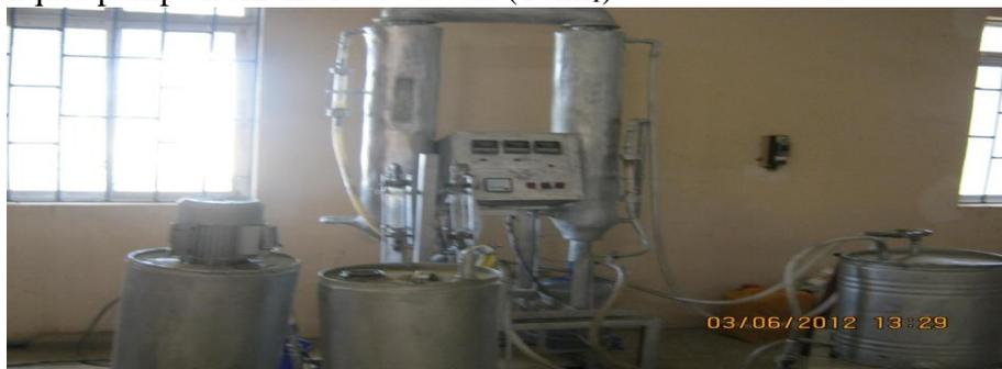
Fig. 1: Continuous Oscillatory Baffled Reactor Arrangement (COBRA)
