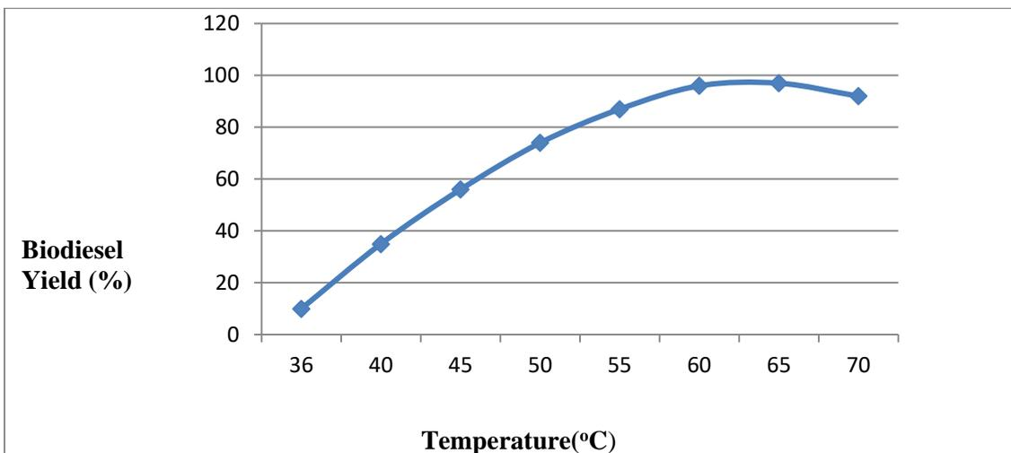
**Fig. 3 : Effect of Temperature on Biodiesel Yield from *Jatropha* oil using ZnO (15w/w% oil)**
